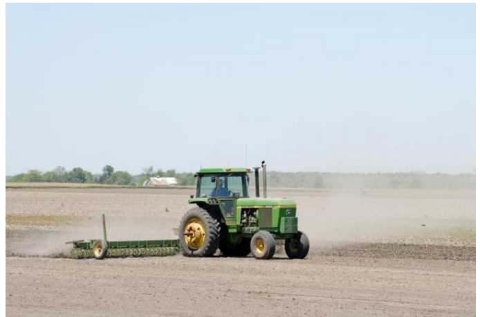
Figure 2. A rotary hoe can dislodge small weeds in a growing crop.
